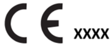
*2 XXXX = Identification number of notified body responsible for the EU type examination and supervising ongoing conformity
